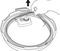
**Removing the gasket:** Pull the rubber gasket from the sides of the inner lid.
