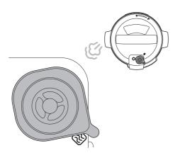
Turn the pressure release value to the CLOSED  $\bigotimes$  position.
