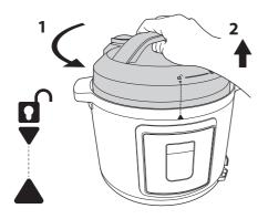
Turn the lid anti-clockwise (1) and then lift off the top of the pressure cooker (2).
