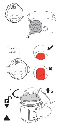
After steam has stopped coming out of the Steam release valve, check that the Float valve has dropped before opening the pressure cookers lid.
