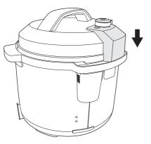
Ensure the tab on the back of the lid slots into the channel on the back of the pressure cooker.
