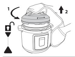
Allow your pressure cooker to cool for a few minutes then undo the lid by rotating it anti-clockwise and lift off.
