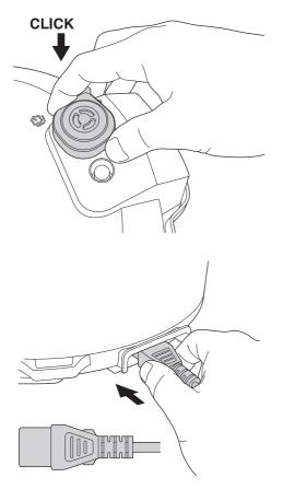
Slot the pressure valve into the large recess on the top of the pressure cookers lid.
