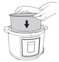
Place the inner pot into the outer body of the pressure cooker.
