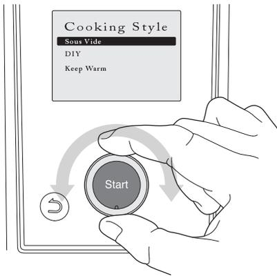
Select the **Sous Vide** program by rotating the control knob then press the **Start** button.
