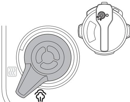
Ensure the pressure release valve is in the
