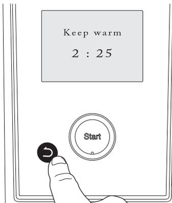
Press the ↶ (back) button to exit the keep warm function.
