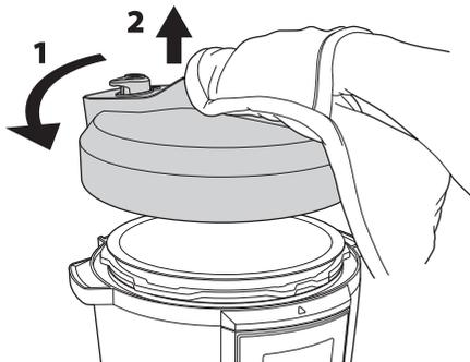
You can now open the pressure cooker's lid by turning the lid anti-clockwise (1) then lifting off upwards (2). Remove the inner pot using a heat proof cloth or oven glove. After using your pressure cooker please clean it by following the Care & Maintenance section of these instructions. **NEVER TOUCH THE PRESSURE VALVE DURING COOKING.**
