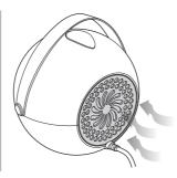
**IMPORTANT:** Ensure that no items can block the air intake on the back of your fan.
