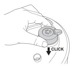
Slot the pressure valve into the large recess on the top of the pressure cookers lid.
