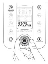
You can now adjust the temperature and the cooking time to your liking by turning the Control Knob clockwise to increase or anti-clockwise to decrease.
