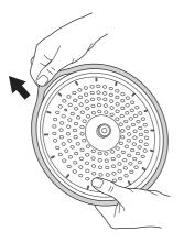
Removing the gasket: Pull the
