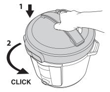
Fit the lid and close by turning it anticlockwise until it locks with a click.
