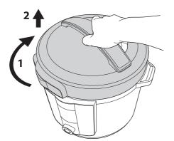
**IMPORTANT: Never fit the lid when using the fry function.** If the lid is properly fitted in place, the FRY function cannot be selected.
