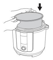
Place the inner pot into the outer body of the pressure cooker.
