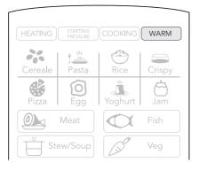
When the timer has finished, your pressure cooker will sound a 'BEEP' and enter the KEEP WARM function, WARM will be highlighted on the display.
