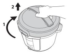
You can now open the pressure cookers lid by turning it clockwise and lifting off. Remove the inner pot using a heat proof cloth or oven glove. After using your pressure cooker please clean it by following the Care & Maintenance section of these instructions. **NEVER TOUCH THE FLOAT VALVE DURING COOKING OR IMMEDIATELY POST COOKING**.
