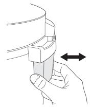
**Condensation cup:** On the back of the steamer under the hinge you will find the condensation cup.
