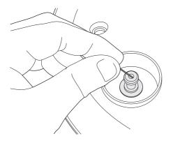
Use a pin to remove any blockages inside or around the valve.
